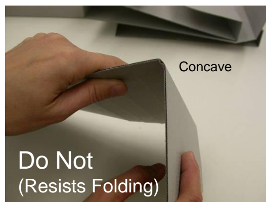
Fig. 6: Do not fold away from concave side
